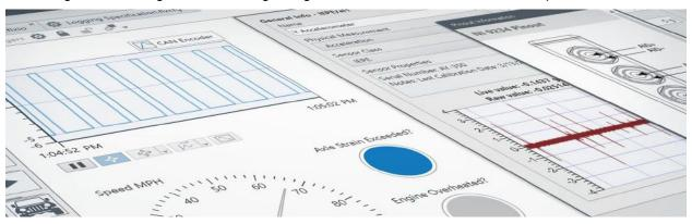
FlexLogger automatically saves metadata documenting your test configuration, so you can quickly trace test results and make comparisons across multiple tests. You can interactively review test results in the integrated data viewer to visually inspect your data and draw conclusions.
