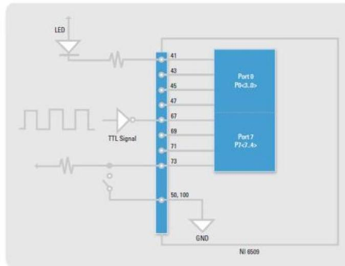
Figure 2. Signal Connections
