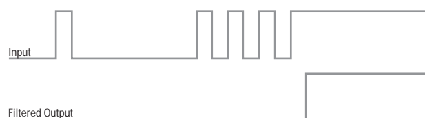
Figure 2. Debouncing and Glitch Removal
