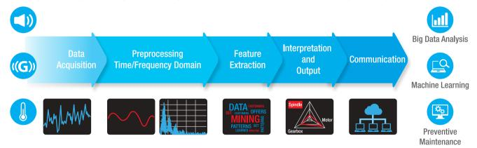
**Data Acquisition:** defines trigger-capture conditions, number of channels, amplification, sampling rate, and conversion of physical phenomena.
