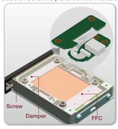
Advantech DLoG responds to the problems associated with electronic systems operating in harsh vehicle environments by thorough research and design. Quality Assurance personnel physically test products in the environments in which they will be used. The development and testing that is conducted follow SAE J1455 4.9.4.2, and MIL-STD-810G 514.5 , and EN60721-3-5 class 5M3 standards.
