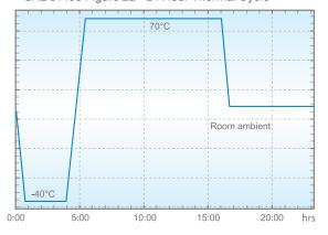
SAE J1455 Figure 2b - Short (8 Hour) Thermal Cycle
