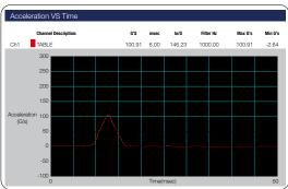
EN 60721-3-5 Class 5M3 Shock Test – Level II (100G /6ms)
