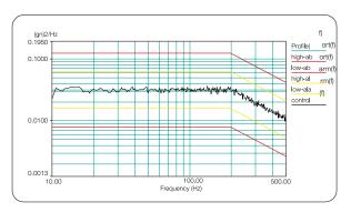
EN 60721-3-5 Class 5M3 Random Vibration Test (3.38Grms) 10~500Hz, 3.38Grms, 1hr/per axis
