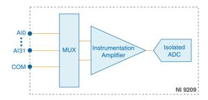
Input signals are scanned, buffered, conditioned, and then sampled by a single ADC.
