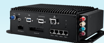
TREK-50N Rugged AI Computer (NVIDIA® Jetson™)
