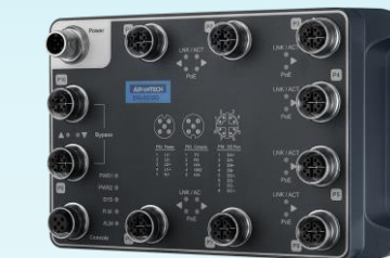
EKI-9520H 20-Port L2 Managed (PoE) Switch w/10G
